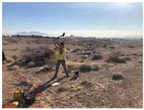
Seismic refraction tomography (SRT) & multichannel analysis of surface waves (MASW) surveys to detect a fault under a caliche layer.
