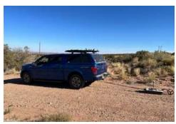
Vehicle towed surveys to map the boundaries of old waste disposal cells using a Geosensors R6 EM instrument and Impulse Radar Raptor-45 real-time sampling GPR array. By using vehicle-mounted instruments we were able to acquire data about 5 times faster than if we were to do the survey of foot.
